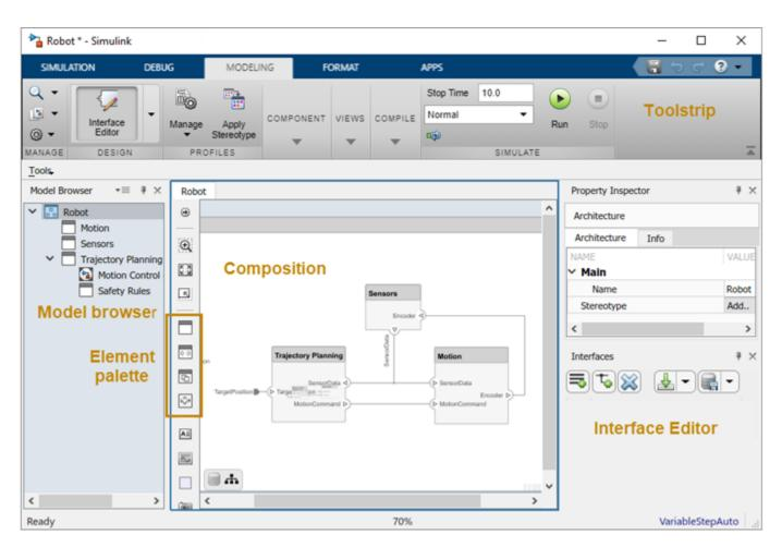
This example shows a motion control architecture, where a sensor obtains information from a motor, feeds that information to a controller, which in turn processes this information to send a control signal to the motor so that it moves in a certain way. You can start with this rough description and add component properties, interface definitions, and requirements as the design progresses.
